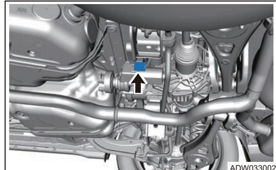
5. Remove 4 fixing bolts between motor and rear final drive.
