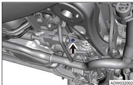
3. Fill new SAF Carbon Mod oil from oil filler until oil level reaches the bottom of filler plug hole.
