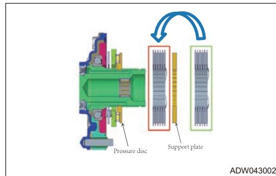
10. Replace new lining set (including 6X outer lining, 5X inner lining and 6X wave spring).
