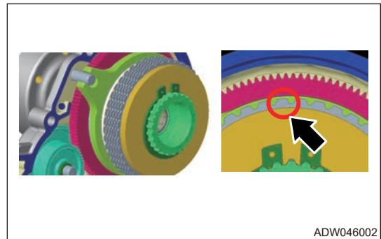
14. Install clutch assembly to rear final drive, tighten 5 fixing bolts (arrow) (preload is  $10 \pm 2 \text{ N}\cdot\text{m}$ , and then continue to rotate  $90^\circ \pm 5^\circ$ ).
