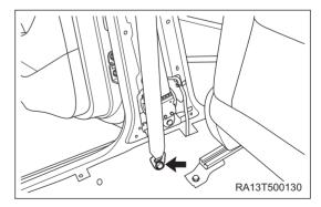
Using a screwdriver wrapped with protective tape, pry off the front seat belt assembly upper bolt cover (arrow).
