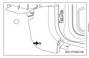
b. Using an interior crow plate, pry off the clip from Apillar lower protector assembly and remove the right A-pillar lower protector assembly (1).
