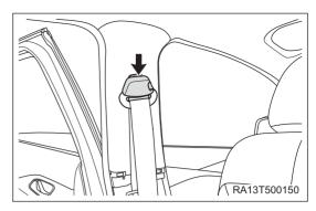
d. Remove the front seat belt assembly upper bolt (arrow) and B-pillar upper protector assembly.
