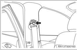
e. Using a screwdriver wrapped with protective tape, pry off fixing clip from B-pillar upper protector and remove B-pillar upper protector.
