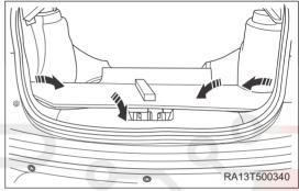
c. Lift up the band in center of the rear part of luggage compartment carpet and remove the luggage compartment carpet assembly by pulling it outward.
