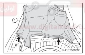
b. Remove 6 clips (arrow) from luggage compartment wheel house assembly and remove the luggage compartment wheel house assembly (1).
