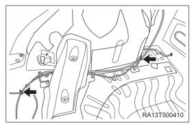
d. Press the claws in the direction of arrow as shown in the illustration, and remove the fuel filler door cable assembly.
