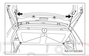
c. Remove the tonneau cover assembly.
