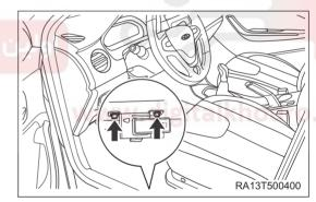
b. Disengage the fuel tank cap cable from slot (arrow) to separate the fuel tank cap cable from fuel tank cap opener assembly.
