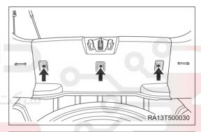
b. Using an interior crow plate, pry off the clips from luggage compartment doorsill pressure plate assembly and remove the luggage compartment doorsill pressure plate assembly (1).
