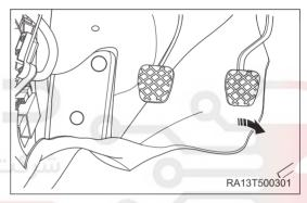
b. Remove the driver side foot rest bracket (arrow).
