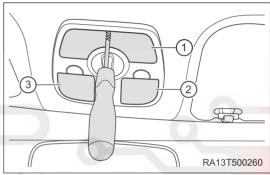
b. Remove 3 fixing screws (arrow) from interior front dome light assembly.
