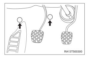
b. Remove the fixing nut (arrow) from the front right side of front floor carpet assembly and remove the front floor carpet assembly.
