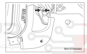
b. Remove the bolt (arrow) from A-pillar lower protector assembly and remove the left A-pillar lower protector assembly (1).
