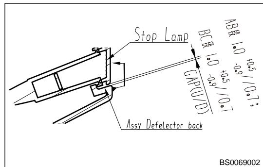
60. Assembly clearance between spoiler assembly and rear windshield.
