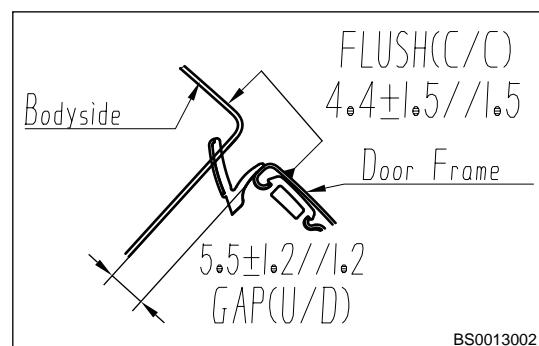
13. Assembly clearance between rear door window frame and front door window frame.
