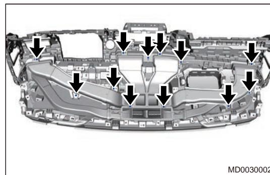
2. Remove the central air duct.
