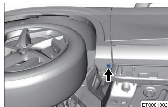
c. Using an interior crow plate, pry off fixing clip from rear left wheel arch.
