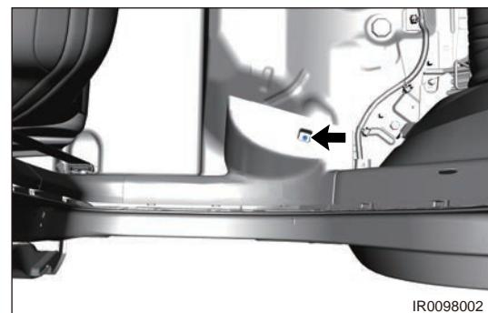
b. Using an interior crow plate, pry off fixing clips from rear left doorsill pressure plate assembly.
