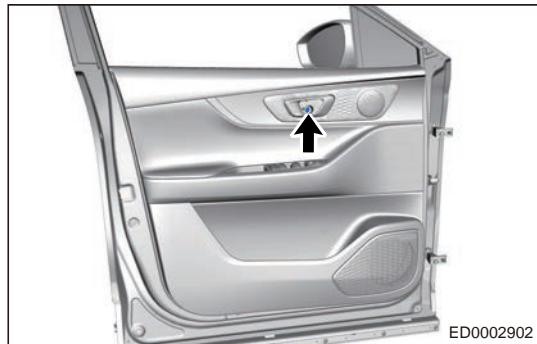
b. Remove 1 fixing screw (arrow) from door protector.
