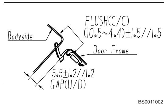
11. Assembly clearance between roof trim strip and front windshield with strip.
