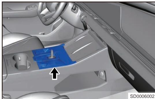
6. Disconnect 2 wire harness connectors (arrow) from auxiliary fascia console control panel.
