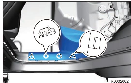
c. Remove the rear left doorsill pressure plate assembly.
