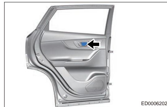
a. Remove 1 fixing screws (arrow).
