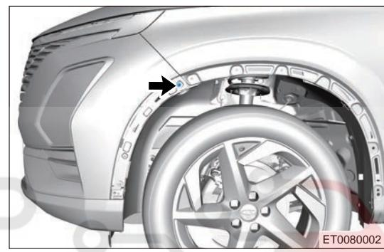
b. Remove fixing screw (arrow) from right side of front bumper.
