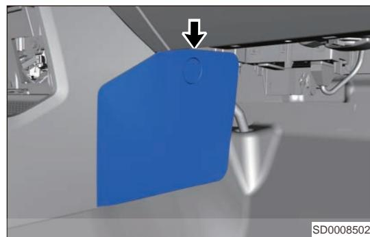
26. Remove 1 fixing bolt (arrow) from the auxiliary fascia console front left end (same to the right).
