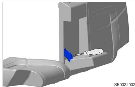
b. Remove center armrest assembly (1) in direction of arrow as shown in illustration.
