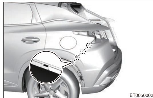
h. Disconnect wire harness connector (arrow) from rear bumper.
