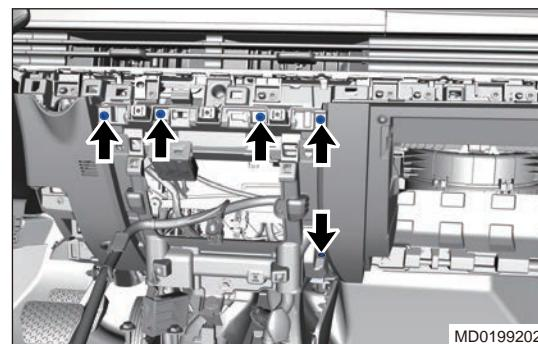
22. Remove 1 fixing bolt (arrow) from center lower protector assembly.
