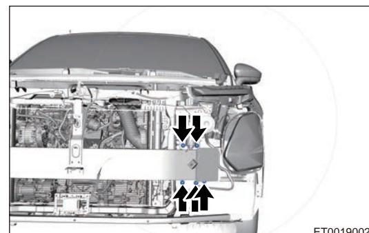
c. Remove 5 fixing nuts (arrow) from left side of front bumper crossmember assembly.
