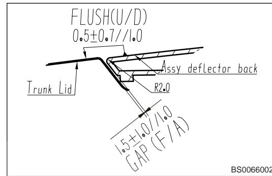
57. Assembly clearance between roof cover and back door.
