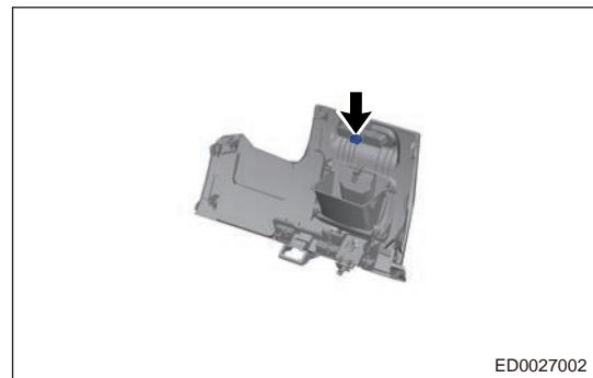
c. Remove the power back door instrument cluster switch assembly.
