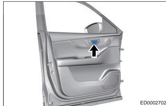
a. Remove the inside handle box cover gasket (arrow).
