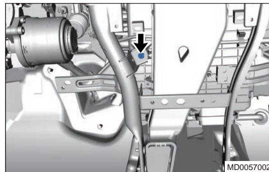
25. Remove 1 fixing screw (arrow) from front part of rear face air duct.
