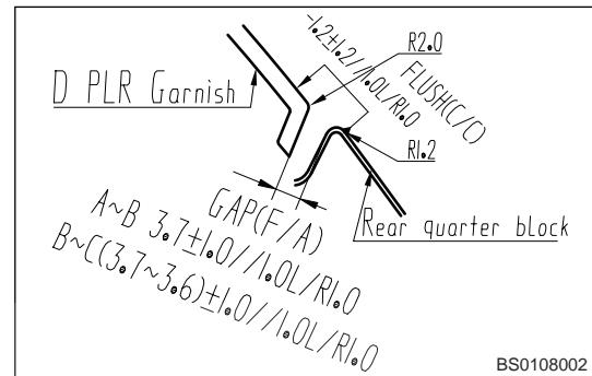
96. Assembly clearance between rear door glass outer weather bar and rear side window glass assembly.
