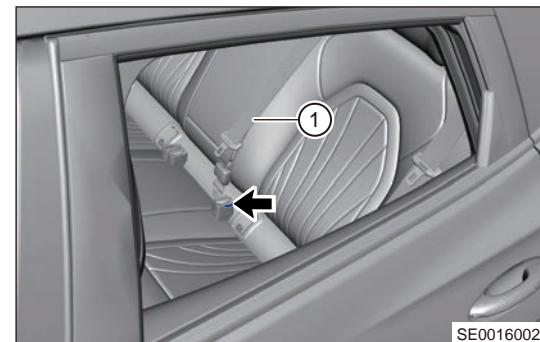
b. Press rear seatback switches (1) and put down rear seat.
