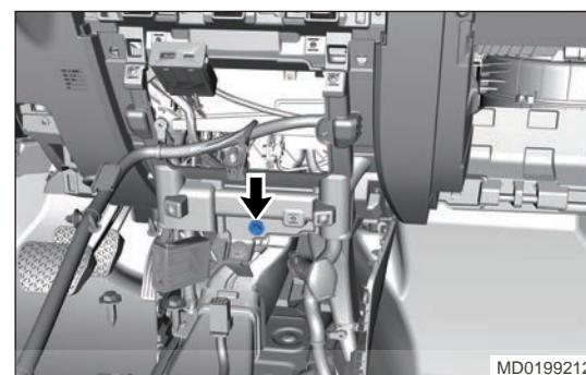
23. Remove 1 fixing clip (arrow) from center lower protector assembly.
