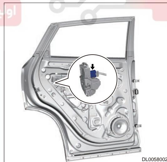
8. Disengage the outside push rod (arrow) from the clip of rear door handle base.
