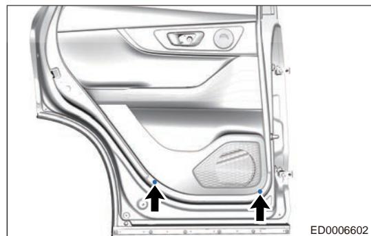
e. Using an interior crow plate, pry up clips on rear door inner protector assembly, and remove rear door inner protector assembly in direction of arrow.
