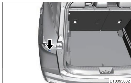
e. Remove 1 fixing bolt (arrow) from upper part of rear bumper assembly.
