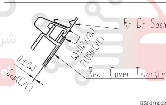
16. Assembly clearance between rear door glass outer weather bar and rear quarter window weather bar.
