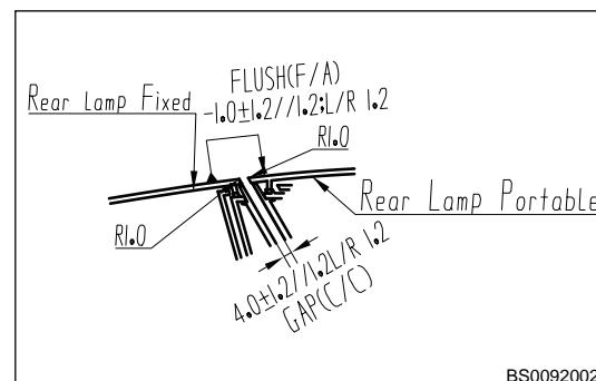
83. Assembly clearance between quarter outer panel and combination light (fixed).
