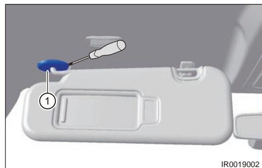
b. Detach sun visor assembly (1) from one side of the holder B, and remove 2 fixing screws (arrow) from left sun visor.
