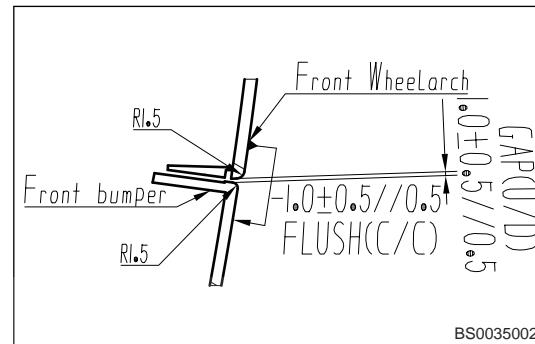
35. Assembly clearance between front bumper upper body and front bumper lower body.
