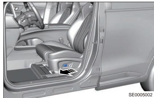
d. Remove 2 fixing bolts (arrow) from rear side of seat assembly.
