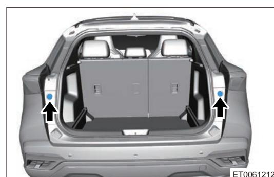
c. Remove 2 fixing screws (arrow) from the rear bumper assembly.
