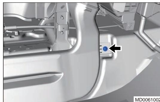
29. Fold back the front passenger carpet to remove fixing screw (arrow) from right foot duct and take away the right foot duct.
