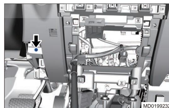
25. Remove 1 fixing bolt (arrow) from the left side of center lower protector assembly.
