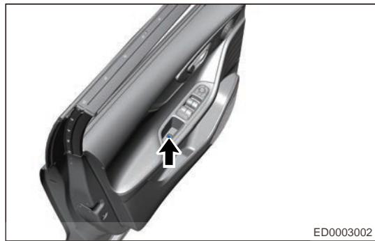
c. Remove 2 fixing screws (arrow) from bottom of door protector.
