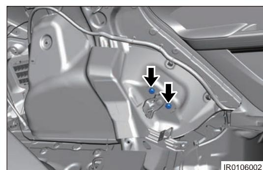
d. Remove the rear seatback left connecting bracket assembly.
