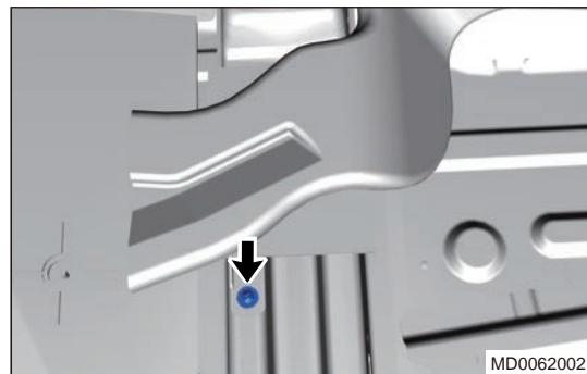
30. Remove 2 fixing bolts (arrow) from instrument panel crossmember fixing bracket (take left side as an example).
