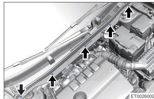
d. Disconnect front washer pipe 1 and remove front windshield lower trim board assembly.
