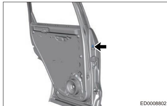
b. Remove fixing bolt (arrow) between rear door lower hinge assembly and rear door assembly.
