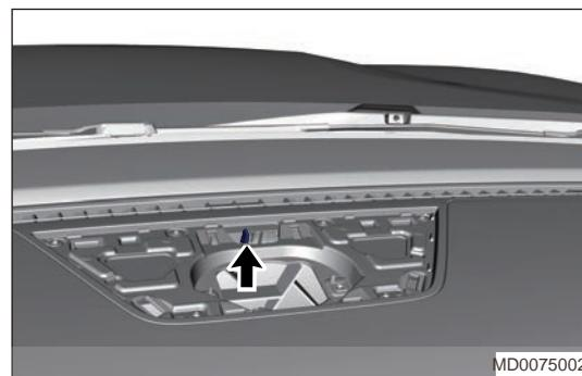
38. Remove the instrument panel assembly.
