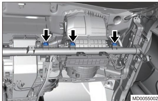
23. Remove fixing bolt (arrow) between HVAC assembly and instrument panel crossmember.
