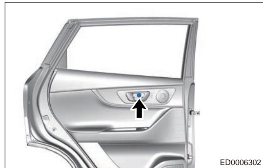
b. Remove the inside handle box cover gasket (arrow).
