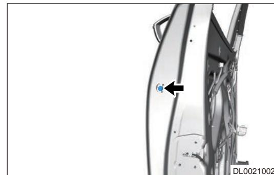
8. Insert the key into the hole on lock cylinder protective cover and carefully pry the lock cylinder cover or using a screwdriver wrapped with protective tape, disengage the claws (arrow) and separate the front door handle protective cover (1) from front door key cylinder assembly (2).
