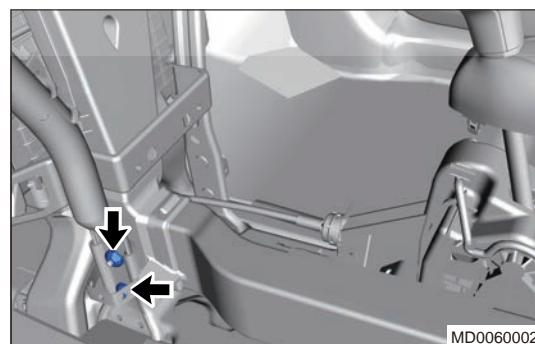
28. Fold back the front passenger carpet to remove 1 fixing screw (arrow) from right foot duct.
