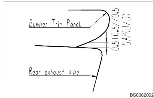
73. Assembly clearance between rear bumper and rear bumper trim panel.
