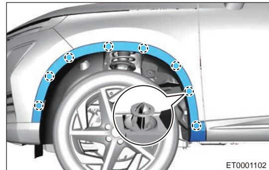
d. Remove the front left wheel arch assembly.
