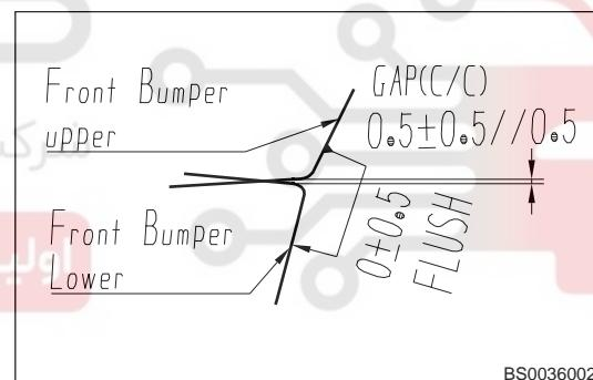
36. Assembly clearance between wing/front bumper and front wheel arch trim panel.
