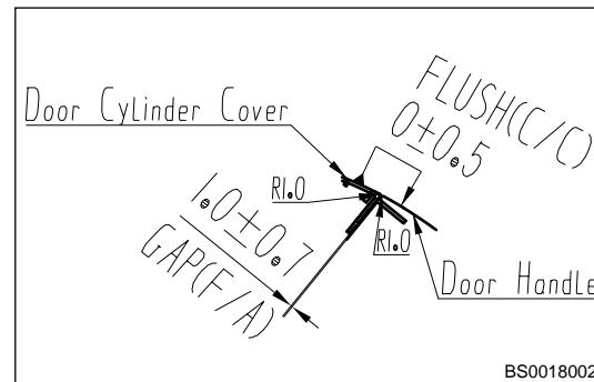
18. Assembly clearance between rear door outer panel and quarter outer panel.
