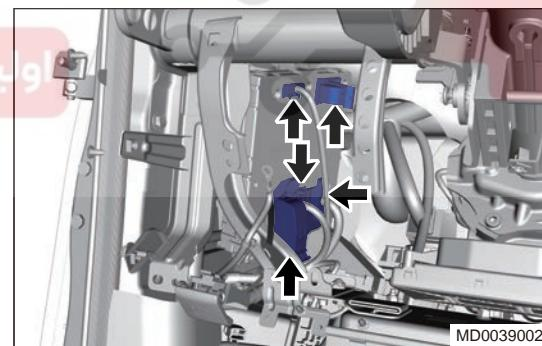
7. Disconnect 5 connectors (arrow) from Body Control Module (BCM).
