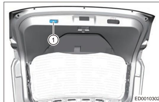
e. Using a screwdriver wrapped with protective tape, pry off claws from back door lower protector assembly.
