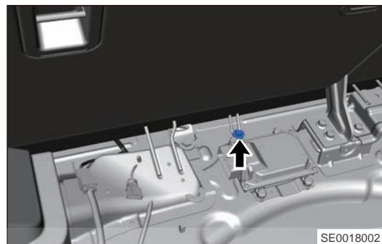
d. Raise up one side of rear seat cushion lightly, and detach fixing clip between cushion and body.
