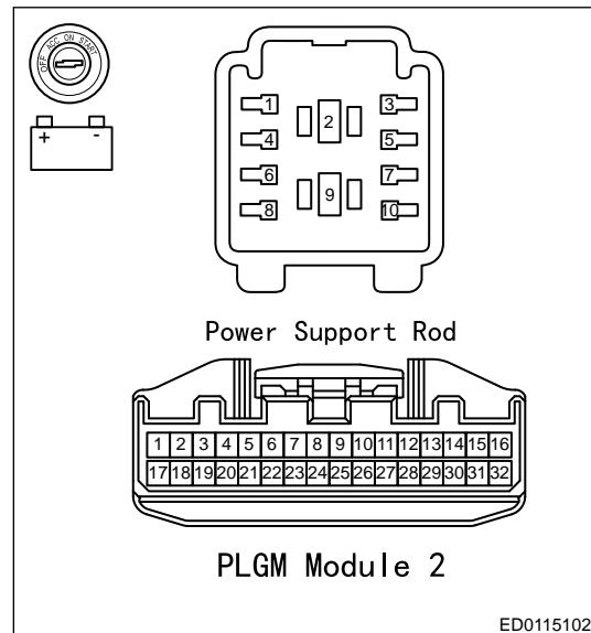
(d) Using ohm band of multimeter, check for continuity between power back door module-2 (227) and power support (1).
