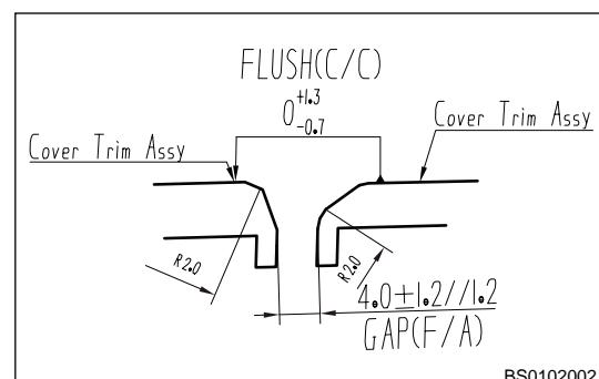
90. Assembly clearance between door trim strip and door cover plate.
