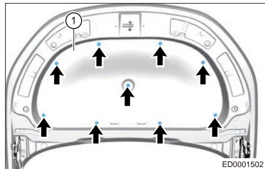
2. Remove the engine hood adjustable buffer block.
