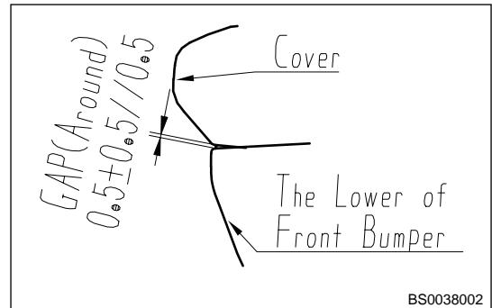
38. Assembly clearance between front bumper body and front bumper lower body.
