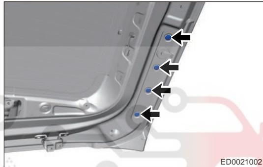
b. Disconnect the anti-pinch strip connector (arrow).
