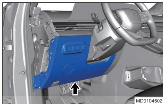
8. Disconnect driving assist switch connector and audio connector (arrow), and remove instrument panel lower left protector assembly.
