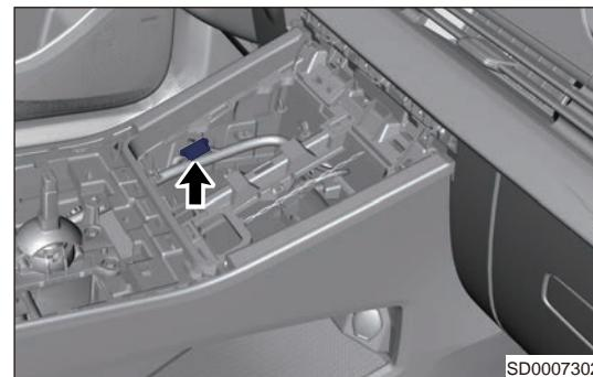
10. Disconnect 1 wire harness connector (arrow) from key induction coil.
