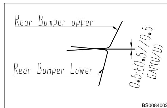
75. Assembly clearance between rear bumper and rear wheel arch.
