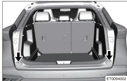
d. Remove 1 fixing bolt (arrow) from upper part of rear bumper assembly.
