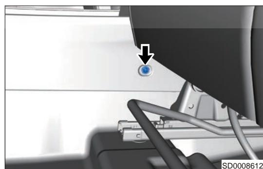
28. Using an interior crow plate, carefully remove the auxiliary fascia console rear panel assembly (arrow).
