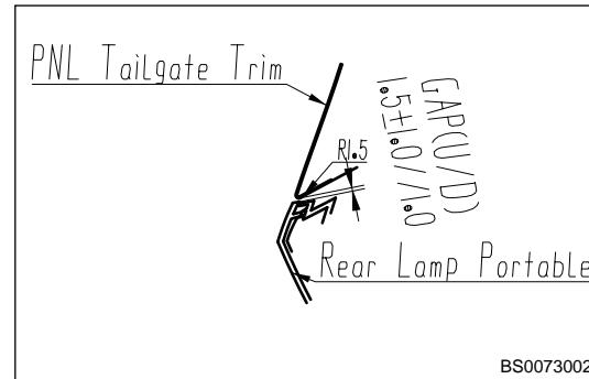
64. Assembly clearance between combination light (- movable) and back door outer panel.
