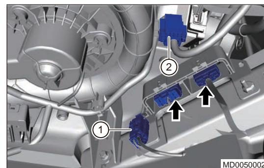
19. Disconnect all wire harness fixing clips (arrow) from instrument panel crossmember.
