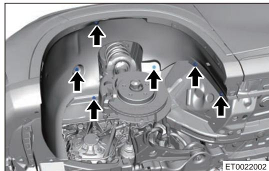
b. Remove 2 fixing screws (arrow) from lower part of front wheel house protector.
