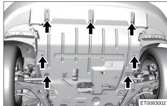
b. Remove 6 fixing snap fasteners (arrow) from engine lower protector assembly.
