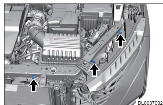
6. Disengage fixing clips (arrow) of engine hood cable assembly.
