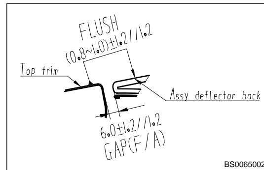
56. Assembly clearance between back door outer panel and spoiler.
