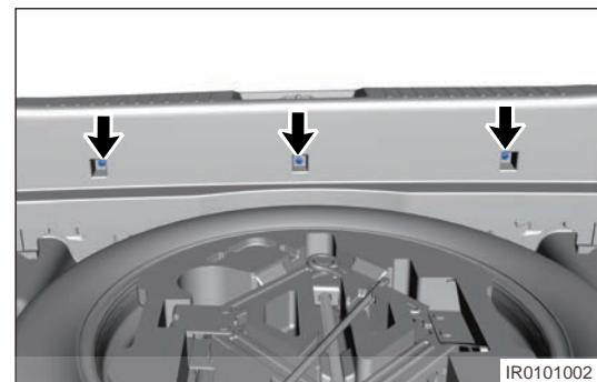
d. Using an interior crow plate, pry off fixing clip from back doorsill pressure plate assembly.
