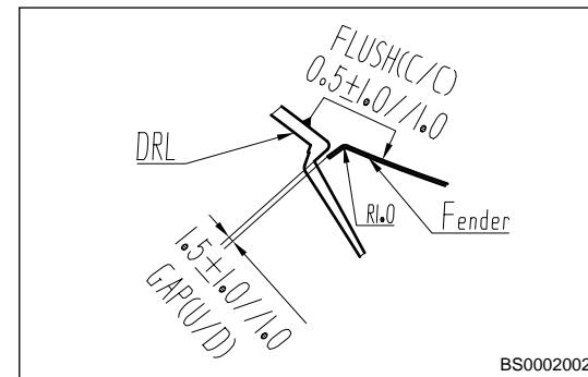
2. Assembly clearance between engine hood and wing.
