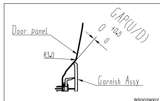
29. Assembly clearance between front door outer panel and engine hood.
