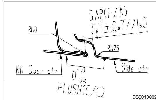
19. Assembly clearance between rear door trim panel and rear wheel arch trim panel.
