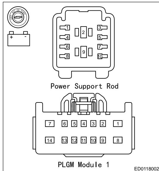
(d) Using ohm band of multimeter, check for continuity between power back door module 1 (104) and power support (2), power back door module 1 (11) and power support (9) and check if there is open.
