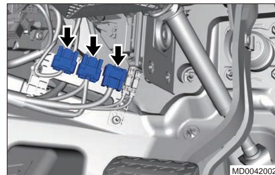
16. Fold back the front passenger carpet to remove instrument panel wire harness body ground nuts (arrow) and disconnect low frequency antenna connector (1).
