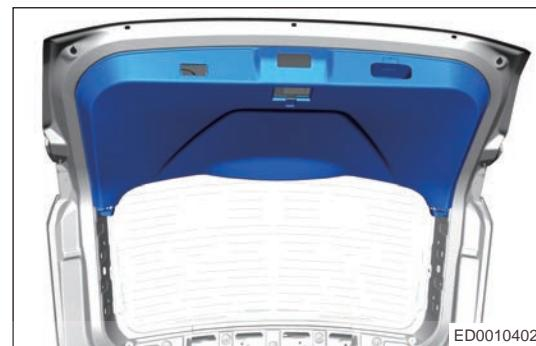
f. Remove the back door lower protector assembly.
