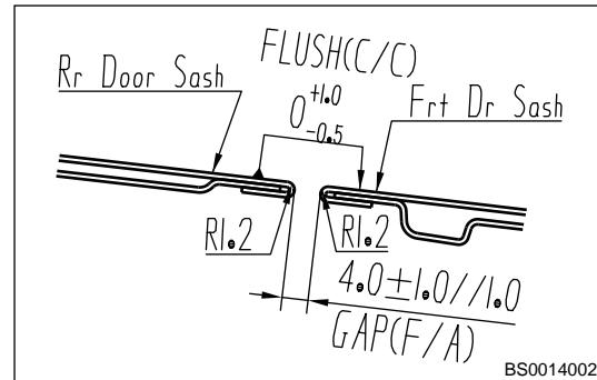
14. Assembly clearance between rear door window frame and rear quadrangular block.
