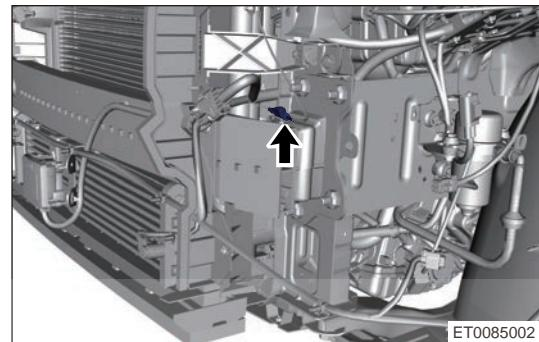
j. Disconnect wire harness connector (arrow) from front bumper radar assembly.
