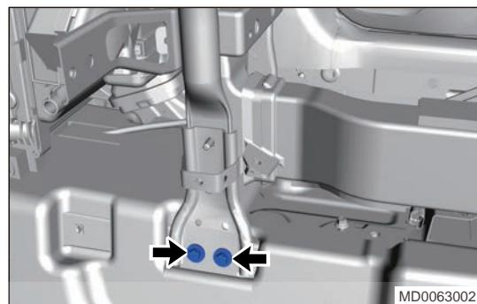
31. Remove fixing bolt (arrow) between HVAC assembly and body.
