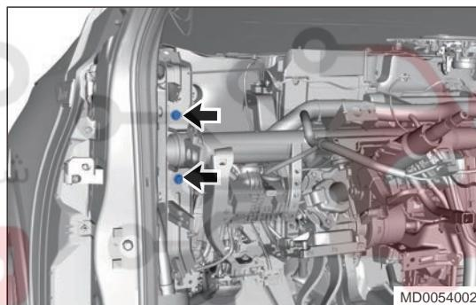
22. Remove 3 fixing nuts (arrow) between HVAC assembly and instrument panel crossmember.
