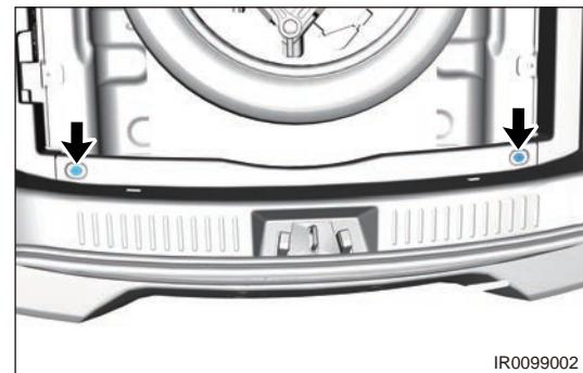
c. Remove 3 fixing screws (arrow) from back doorsill pressure plate assembly.
