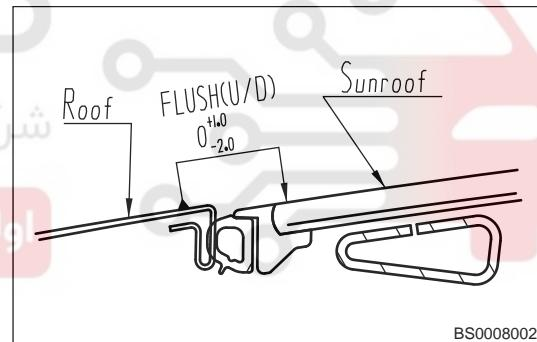
8. Assembly clearance between roof and roof cover.
