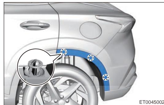
c. Remove the rear left wheel arch assembly.
