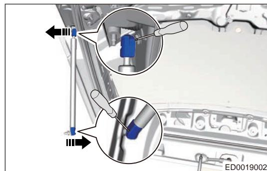
d. Remove the power support assembly in direction of arrow.
