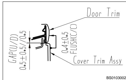
91. Assembly clearance between front door trim strip and rear door trim strip.
