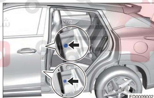
b. Remove 2 fixing bolts (arrow) between front door lower hinge assembly and quarter.
