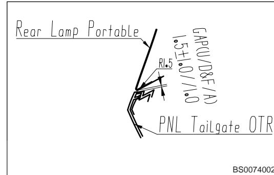
65. Assembly clearance between back door outer panel and rear bumper body.
