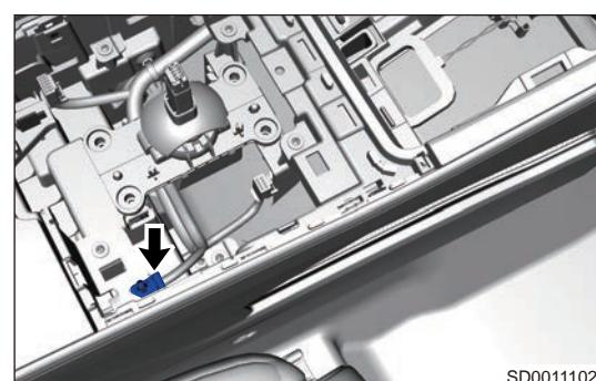
14. Remove 5 wire harness clips (arrow) with interior crow plate.
