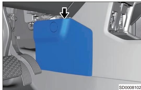
25. Remove the auxiliary fascia console front right end cover plate (arrow).
