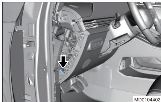
7. Pry up instrument panel lower left protector assembly (- arrow) with interior crow plate.
