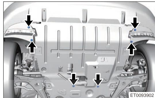
c. Remove the engine lower protector assembly.
