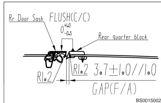
15. Assembly clearance between rear door window frame and rear triangular block window frame.
