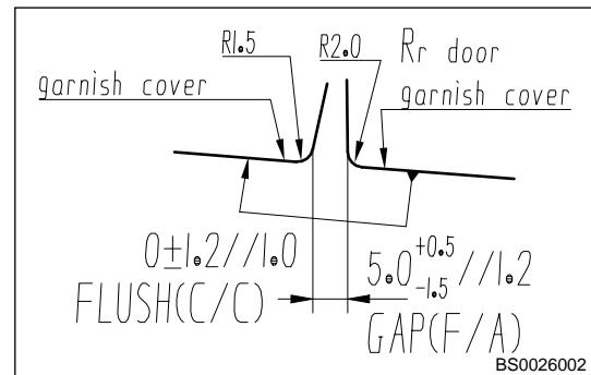
26. Assembly clearance between rear door trim panel and rear door trim panel.
