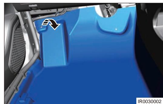
b. Remove fixing clip (arrow) from driver side foot rest.
