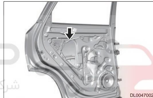
7. Disconnect the connector (arrow) from rear door lock assembly.
