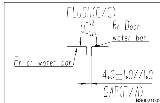
21. Assembly clearance between outer weather bar and door outer panel.
