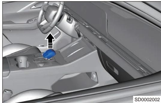
5. Using an interior crow plate, remove the auxiliary fascia console control panel (arrow).
