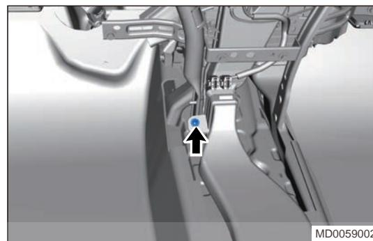
26. Remove 2 fixing screw (arrow) from front part of rear face air duct.
