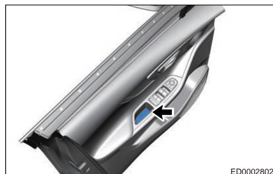
a. Remove 1 fixing screw (arrow) from door protector.
