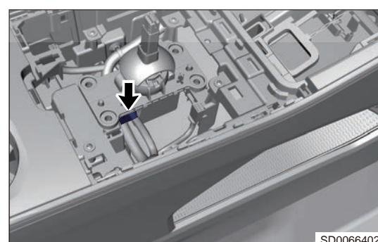
13. Disconnect 1 wire harness connectors (arrow) from auxiliary fascia console.
