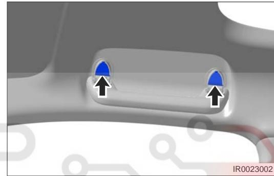
b. Remove 2 fixing screws (arrow) from front right passenger grip assembly.
