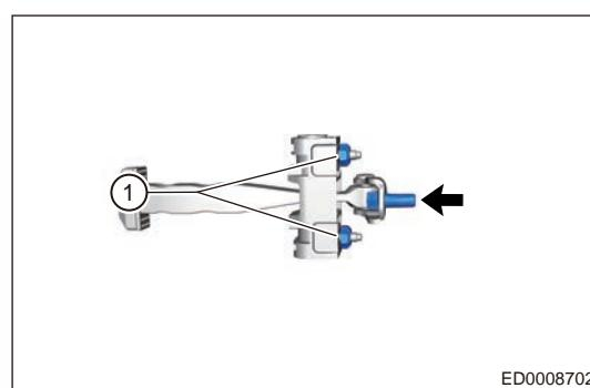
c. Remove rear left door check assembly from door assembly.
