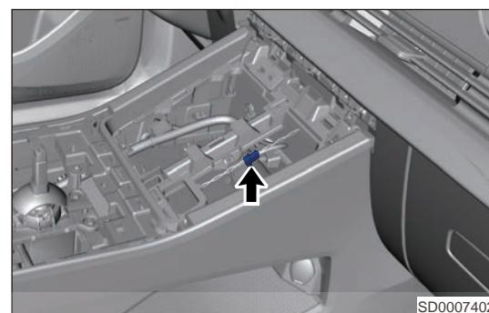
11. Remove 4 fixing bolts (arrow) from electronic shift mechanism.
