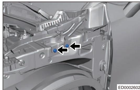
d. Remove the engine hood left hinge assembly.
