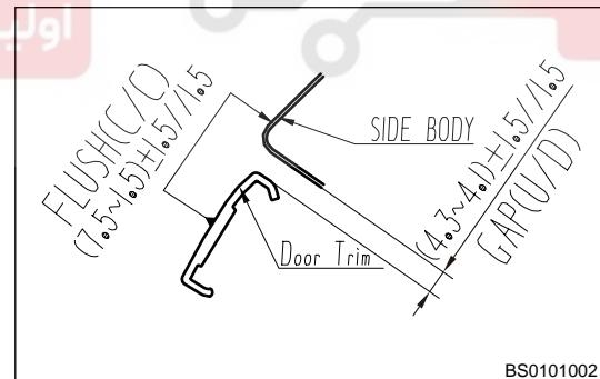
89. Assembly clearance between front door cover plate and rear door cover plate.
