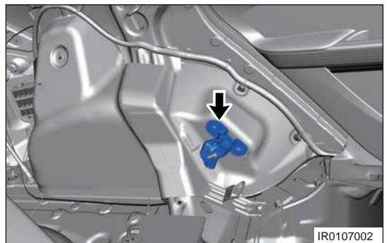
e. Remove the rear wheel house sound insulator assembly (1).
