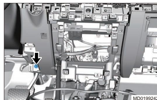
26. Pry up center lower protector assembly with interior crow plate.
