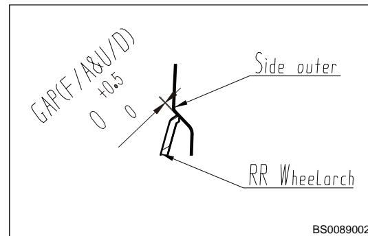
80. Assembly clearance between combination light (fixed) and rear bumper body.
