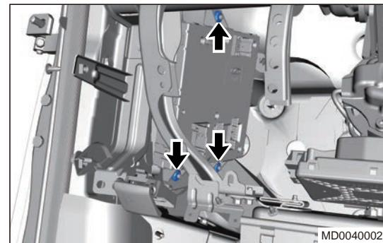
9. Disconnect the wireless communication module connector (arrow).
