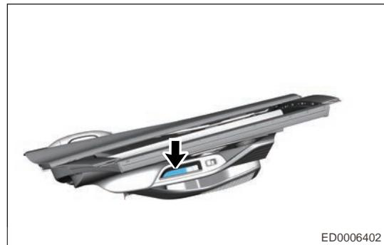
c. Remove 1 fixing screw (arrow) on the rear side of rear door handle box block cover.
