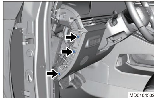
6. Remove 1 fixing bolt (arrow) from instrument panel left end panel assembly.
