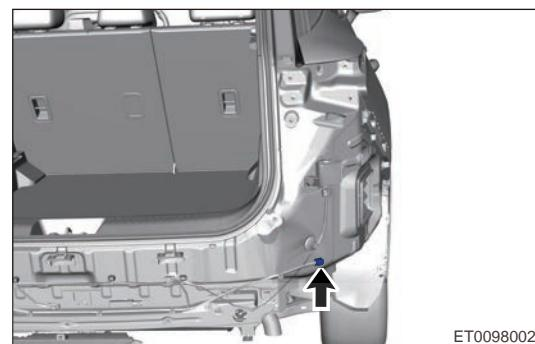
i. Disconnect wire harness connector (arrow) from rear bumper.
