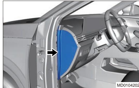
5. Remove 3 fixing screws (arrow) from instrument panel left end panel assembly.
