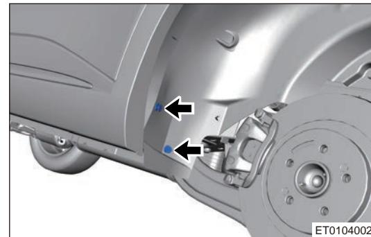
c. Remove 2 snap fasteners (arrow) from rear left wheel house protector assembly.
