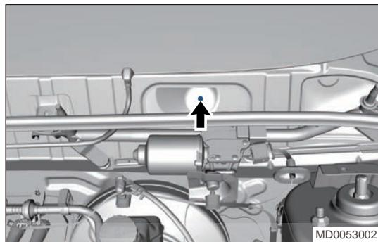
21. Remove 2 fixing bolts (arrow) from instrument panel crossmember (take left side as an example).
