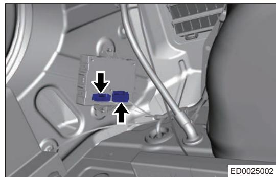
c. Remove the power back door module.
