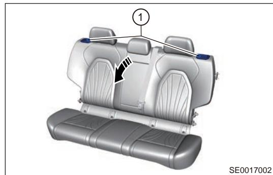
c. Remove fixing bolts (arrow) between rear part of rear seat cushion and body.
