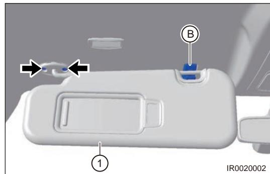
c. Disconnect the left sun visor connector (arrow) and remove sun visor assembly (1).
