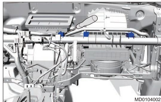
33. Carefully remove the instrument panel crossmember assembly.
