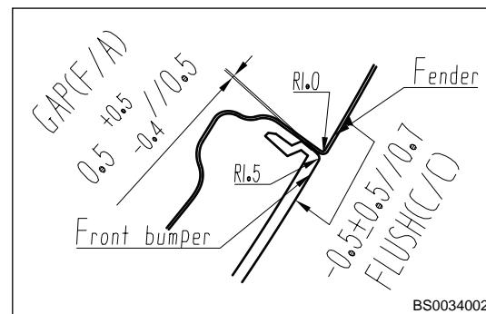
34. Assembly clearance between front bumper and front wheel arch.
