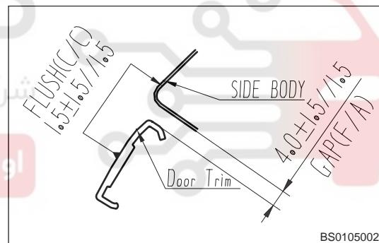
93. Assembly clearance between rear door strip and rear quadrangular trim panel.
