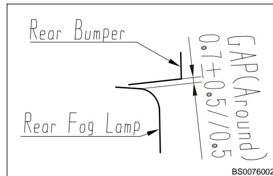
67. Assembly clearance between upper part and lower part of rear bumper trim panel.
