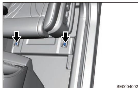
c. As shown in the illustration, press power seat front-back adjustment switch, and move seat assembly to foremost position.
