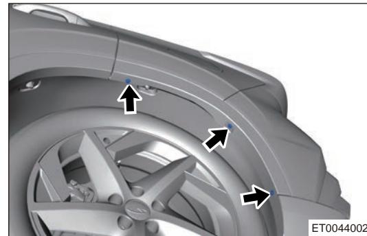
b. Using an interior crow plate, pry off fixing clips from rear left wheel arch.
