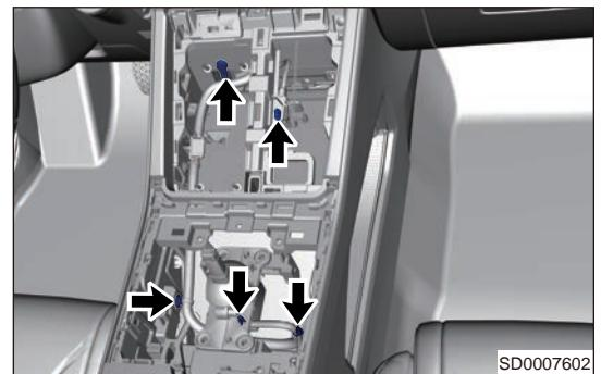
15. Pull the wire harness out from auxiliary fascia console.
