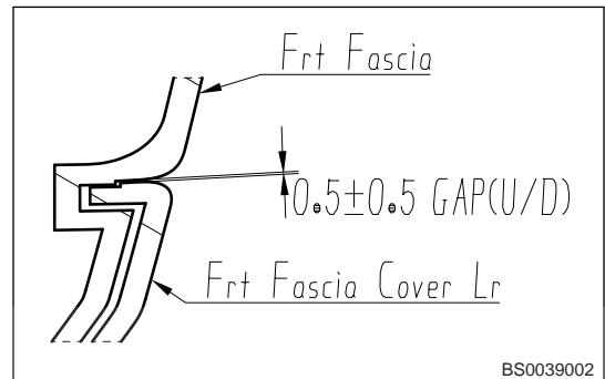
39. Assembly clearance between trim cover and front bumper upper body.
