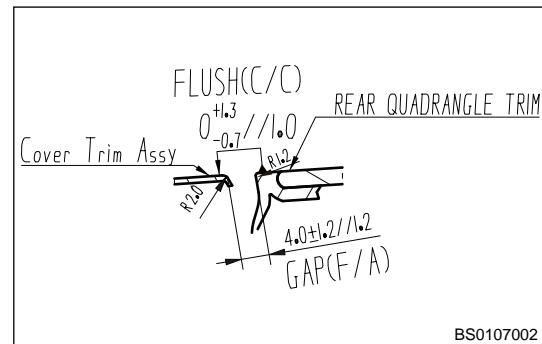
95. Assembly clearance between D-pillar trim panel and rear quadrangular block.
