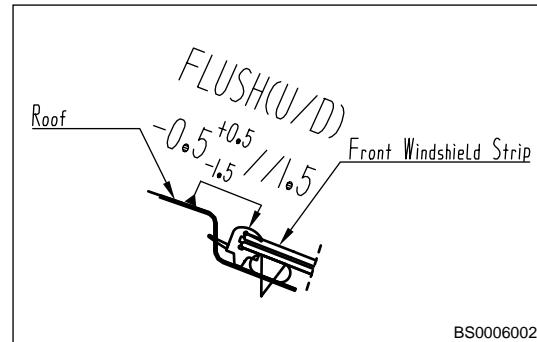
6. Assembly clearance between quarter A-pillar and front windshield strip.
