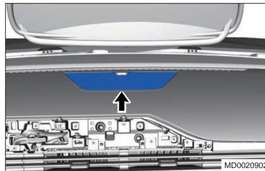
37. Disconnect speaker connector, and remove speaker assembly (arrow).
