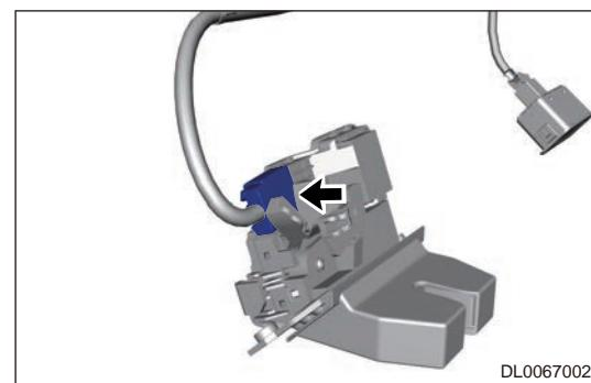
5. Remove 2 fixing bolts (arrow) from back door lock assembly, and remove the back door lock assembly.
