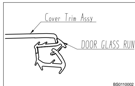
98. Assembly clearance between front door glass outer weather bar and rear door glass outer weather bar.
