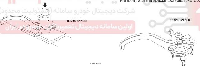
Install the snap ring into the groove of the knuckle.
