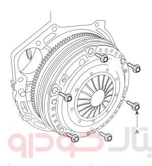
Using the SST(09411-11000), install a disc(A).
