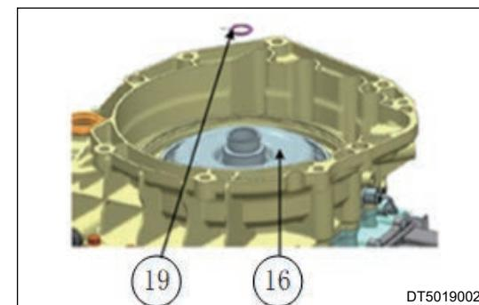
a. Using a clutch measuring fixture, measure the clearance H between end face of clutch and end face of input shaft snap spring groove.
