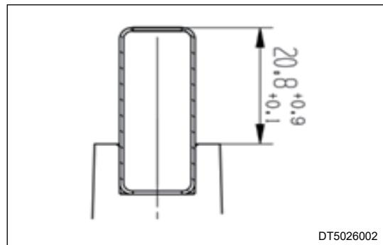
16. Install half shaft oil seal (32) to main housing side.
