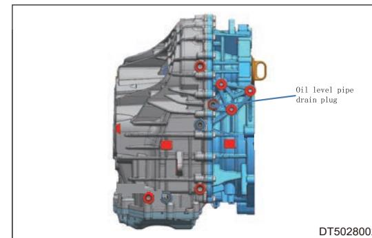
22. When the oil in the drain plug hole flows out with drops, tighten the drain plug.
