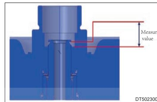
b. Select a appropriate clutch adjusting shim (19) to install to clutch assembly according to the following rules.
