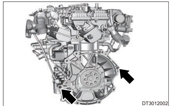
2. Align the dowel pin hole of transmission with the dowel pin hole of engine, push the transmission so that the joint surfaces between engine and transmission can be contacted well, and install 2 coupling bolts (arrow) to engine side.
