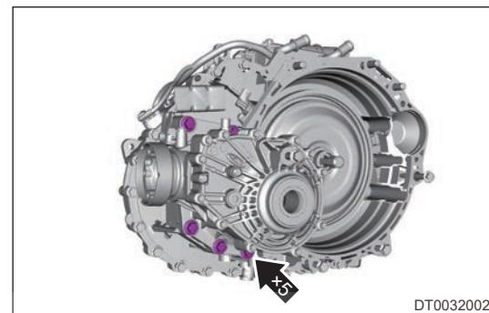
c. Remove the transfer assembly.
