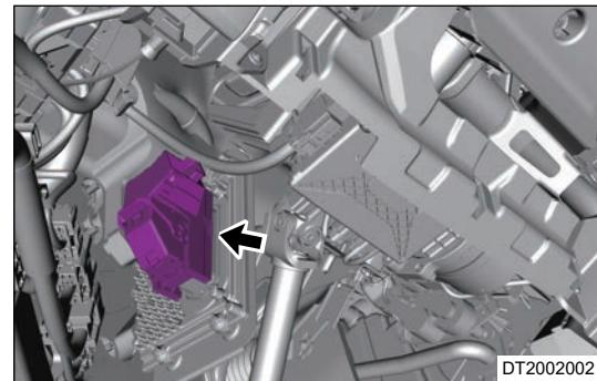
4. Remove 4 fixing bolts (arrow) from transmission control unit.
