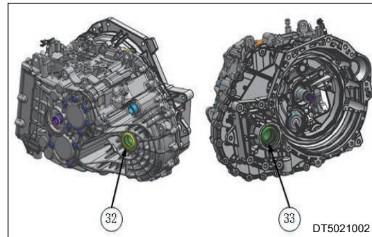
17. Install half shaft oil seal (33) to clutch housing side.
