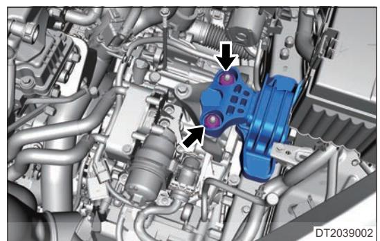
26. Remove 3 fixing bolts (arrow) between upper part of transmission and engine.
