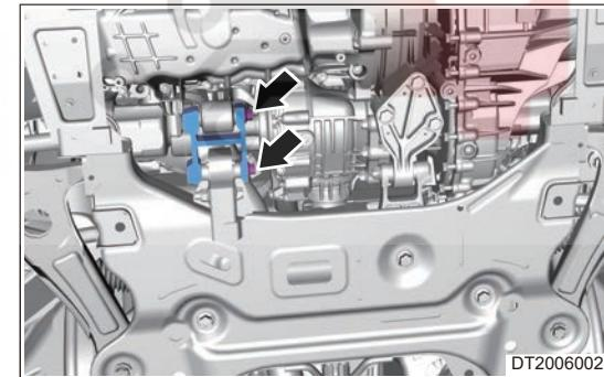
15. Raise vehicle to a proper height, remove front left/right lower impact crossmember.
