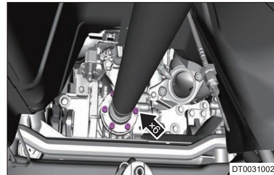
b. Remove 5 fixing bolts (arrow) between transfer and transmission.
