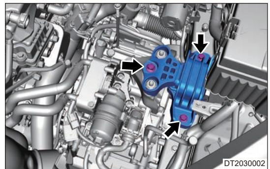
25. Remove 2 fixing nuts (arrow) from left mounting cushion, and remove left mounting cushion.
