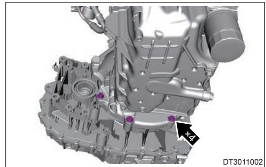
31. Separate transmission and engine assembly, and remove transmission assembly.
