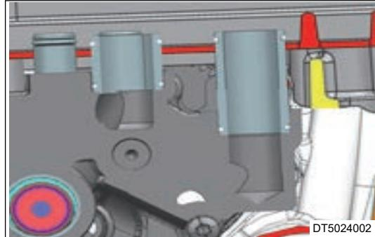
7. Pass transmission wire harness connector assembly (3) through transmission case and install, and then tighten 2 fixing bolts (9) to transmission wire harness connector assembly. Tightening torque: 2 - 3 N·m.
