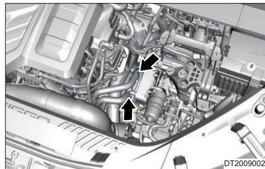
8. Disengage inlet pipe (1) and (2).
