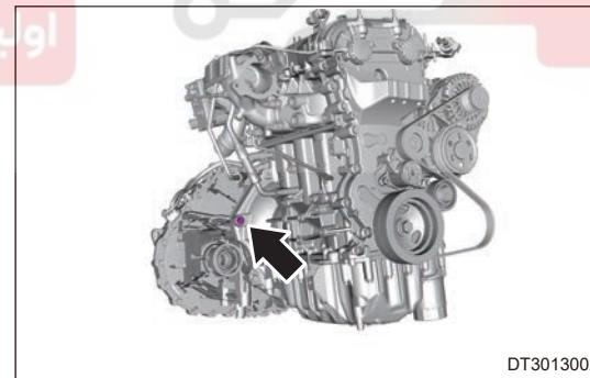
30. Remove 3 fixing bolts (arrow) between lower part of engine and transmission.
