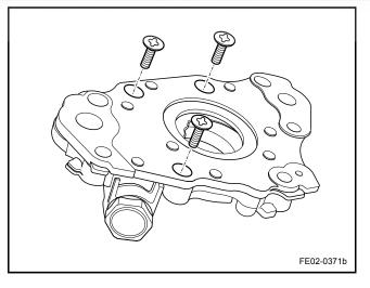
3. Install the oil pump rear cover and tighten connecting bolt.
