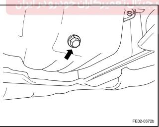
6. Install and tighten oil pan oil discharge bolts.
