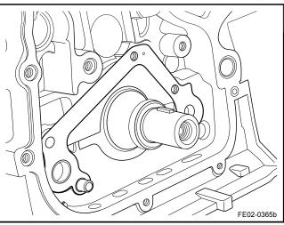
3. Install the oil pump gasket.
