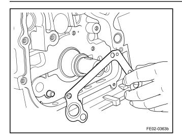
6. Remove the oil pump gasket from the engine block.
