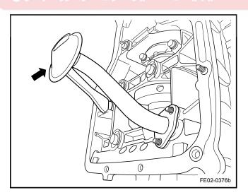
1. Inspect and clean set of filters before installing the oil pan.
