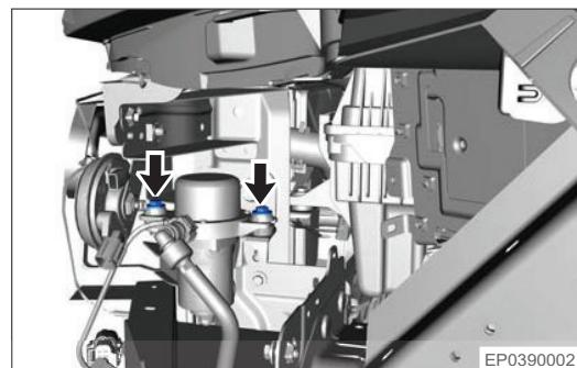
7. Remove the vacuum pump assembly.
