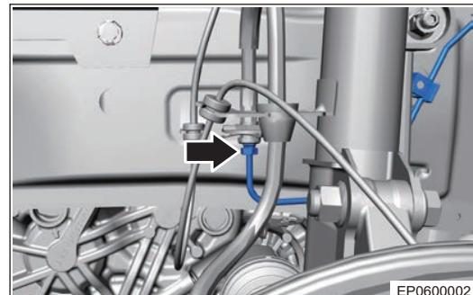
23. Remove the front left brake pipe II assembly.
