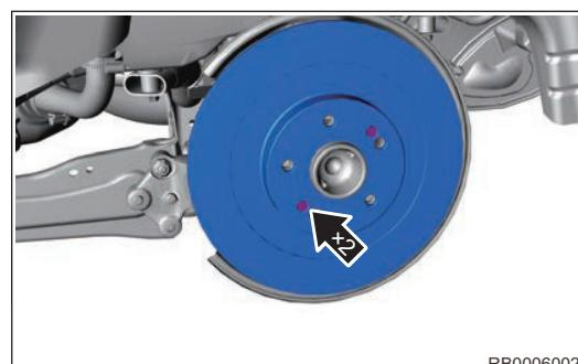
8. Remove the rear brake disc.
