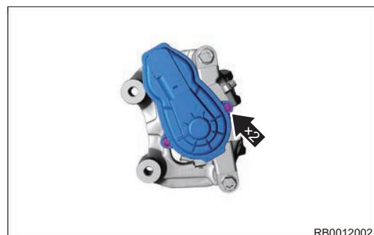
5. Remove the electronic control execution unit.
