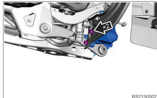
16. Remove the rear left steering knuckle assembly.
