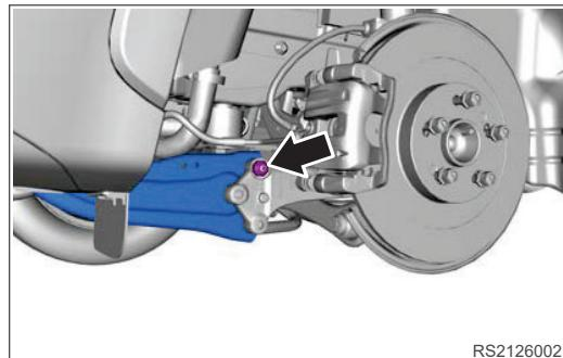
5. Remove 2 coupling bolts between rear left steering knuckle assembly and rear left trailing arm assembly.
