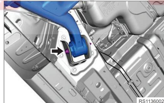
5. Remove 5 fixing bolts (arrow) between rear left shaft bracket and body.
