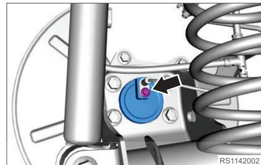
7. Remove 4 fixing bolts between rear hub bearing and rear left steering knuckle.
