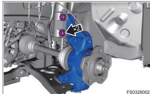
14. Disengage the left drive shaft and remove the front left steering knuckle assembly.
