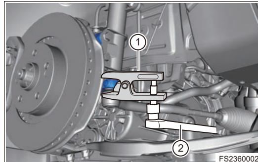
10. Remove fixing bolt between front left wheel speed sensor and front left steering knuckle assembly, and disengage the front left wheel speed sensor carefully.
