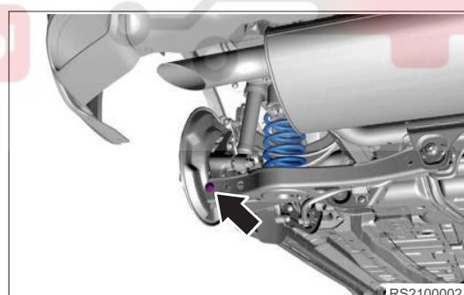
6. Lower the transmission carrier slowly to an appropriate height and remove the rear coil spring carefully.
