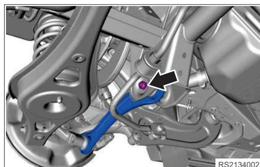
6. Remove the rear left pull rod assembly.
