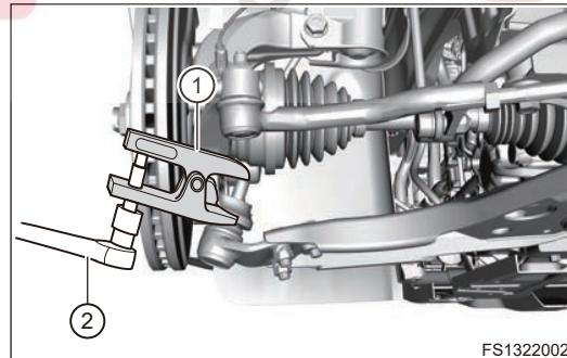
8. Remove fixing nut between left steering tie rod outer ball pin assembly and front left steering knuckle assembly.
