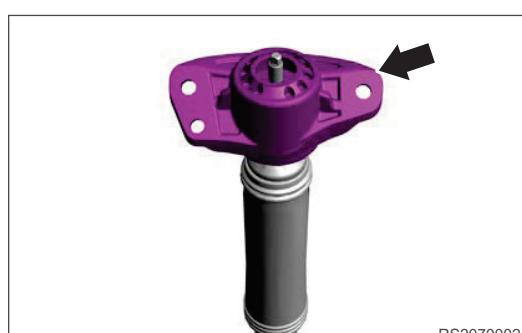
4. Remove the rear buffer block.
