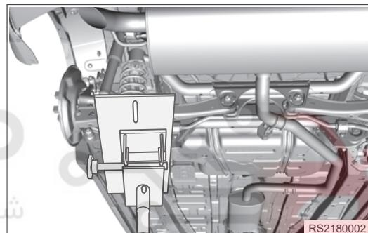
5. Remove coupling bolt and nut between rear lower control arm assembly and rear steering knuckle assembly.
