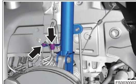
6. Remove 2 coupling bolts and nuts between front left shock absorber assembly and front left steering knuckle assembly.
