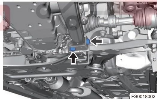
6. Remove nut between front left control arm ball pin and front left steering knuckle.
