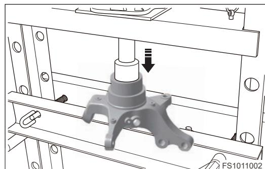
6. Remove the front hub bearing carefully.
