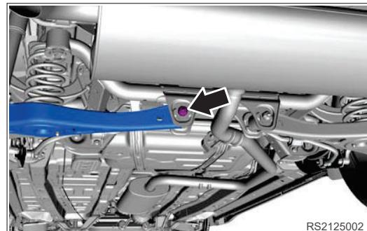
8. Remove the rear left lower control arm assembly.
