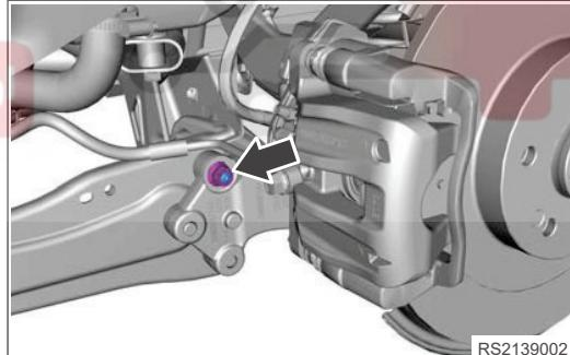
4. Remove coupling nut between rear left connecting rod assembly and rear stabilizer bar assembly, and remove rear connecting rod assembly.
