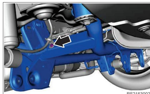
10. Install transmission carrier to support rear sub frame assembly.
