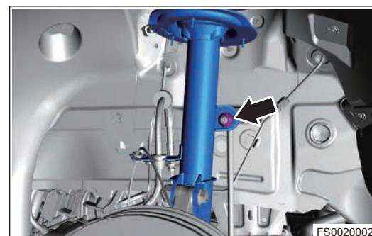
5. Disengage the front left wheel speed sensor wire harness and front left brake hose assembly from front left shock absorber assembly.
