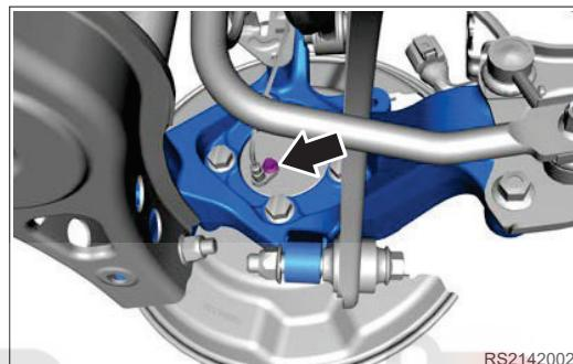
7. Remove 4 fixing bolts between rear left hub bearing and rear left steering knuckle.
