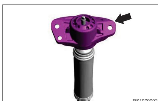
4. Remove the rear buffer block.
