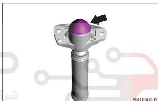
2. Remove fixing nut from rear left shock absorber assembly.
