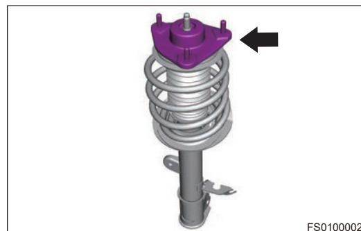
5. Remove bearing assembly from upper part of front left shock absorber assembly.
