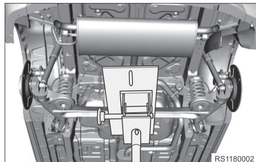
5. Remove coupling bolts and nuts between rear shock absorber assembly and rear shaft assembly.
