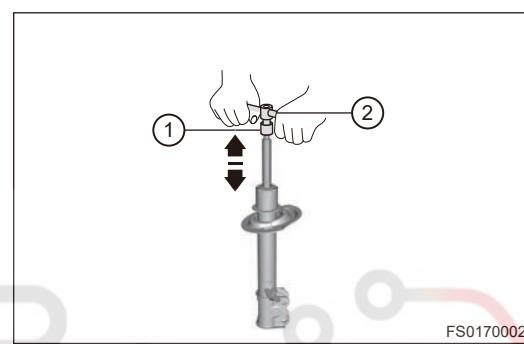
b. Compress and extend front shock absorber strut several times by hands in direction of arrow as shown in illustration. Check that there is no abnormal resistance or unusual sound during operation. If there is any abnormality, replace the front shock absorber assembly with a new one.
