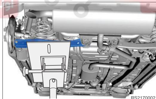
5. Remove coupling bolt and nut between rear left lower control arm assembly and rear left steering knuckle assembly.
