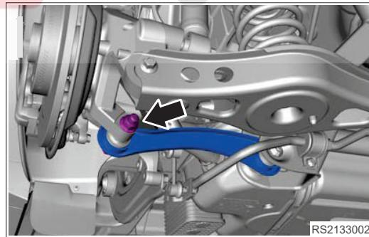
5. Remove coupling bolt and nut between rear left pull rod assembly and rear sub frame welding assembly.
