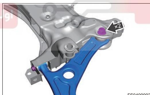
4. Remove the front right control arm assembly.
