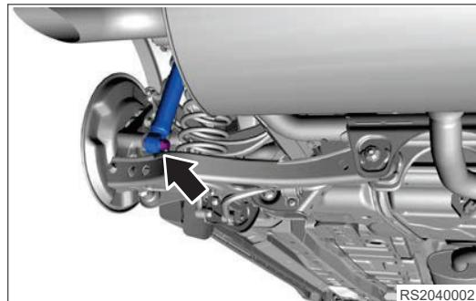
7. Remove the rear left shock absorber assembly.
