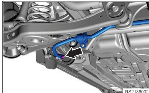
4. Remove 2 coupling bolts between rear stabilizer bar assembly and rear sub frame welding assembly (take left side as an example). Use same removal procedure for right side.
