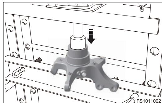
5. Remove the front hub bearing carefully.
