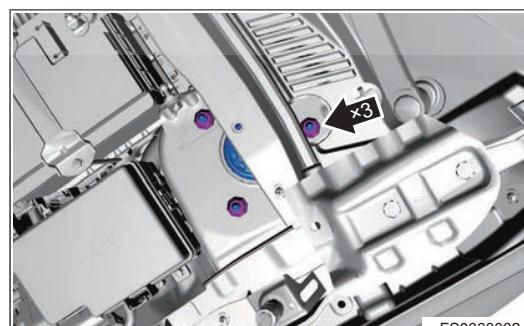
9. Remove the front left shock absorber assembly with front coil spring.
