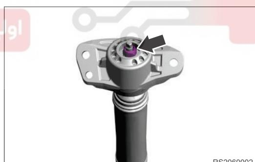
3. Remove the rear left shock absorber upper connecting plate assembly (w/ insulator).
