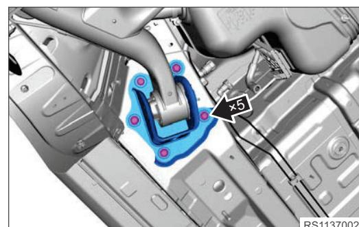
6. Remove the rear left shaft bracket.
