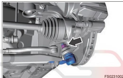
5. Remove 2 fixing nuts and 1 fixing bolt (1) between front left control arm and front left control arm ball pin.
