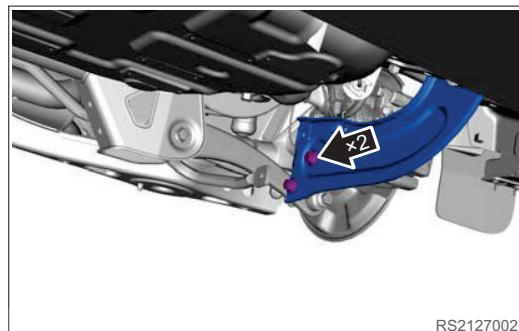
6. Remove 4 coupling bolts between rear left trailing arm assembly mounting bracket and body.
