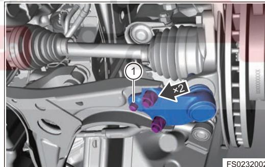
6. Use the ball remover (1), turn the wrench (2) to detach the front control arm ball pin and steering knuckle.
