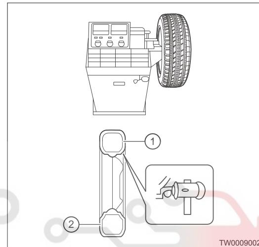
7. Perform test again after assembly is completed, until the balancer displays 0.
