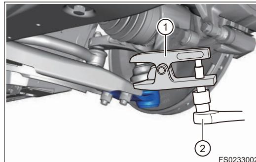
7. Remove the front left control arm ball pin assembly.
