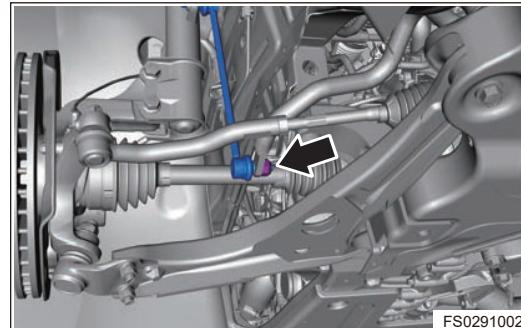
5. Remove coupling nut between front left connecting rod assembly and upper part of front left shock absorber assembly, and remove front left connecting rod assembly.
