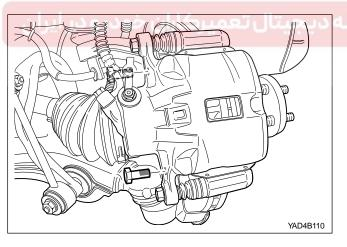
3. Remove the caliper mounting bolt and remove the caliper assembly.
