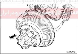
**Notice:** For part-time 4WD, remove the locking hub assembly and hub range before removing the brake disc.
