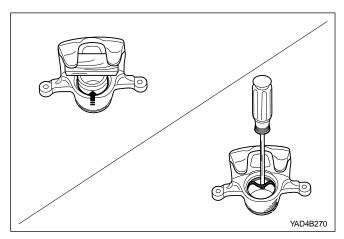
• Using the compressed air, blow out the piston from housing.
