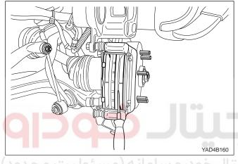
2. Move the caliper cylinder assembly upward and fix it to prevent hose damage.
