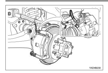
3. Connect the brake hose to the caliper cylinder.
