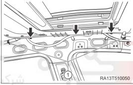
b. Remove 2 clamps (1) from sliding roof right drain hose and sliding roof drain hose joint, and then remove 3 fixing bolts (arrow).
