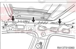
c. Remove 3 fixing bolts (arrow) from front part of sliding roof bracket.
