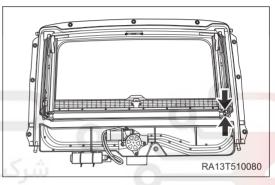
5. Move sliding roof visor assembly in direction of arrow to remove it.
