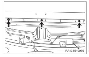
d. Remove the sliding roof bracket.
