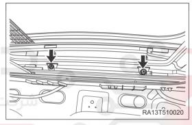
Remove 2 fixing bolts (arrow) from right side of sliding roof glass.
