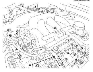
22. After connecting the MAF sensor connector(A) and the breather hose(B), install the air cleaner assembly(C).
