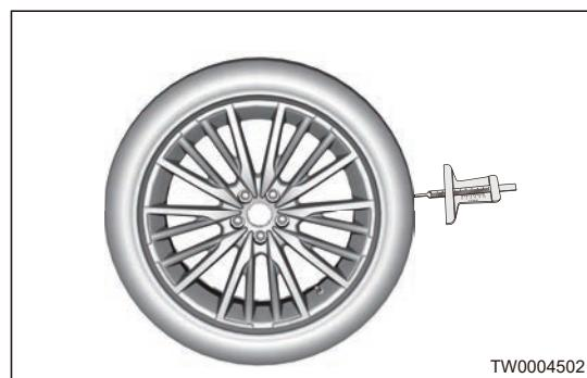
6. Use tire pressure gauge to check if pressures of all tires (including spare tire) are normal. Inflate tires to specified tire pressure as necessary.
