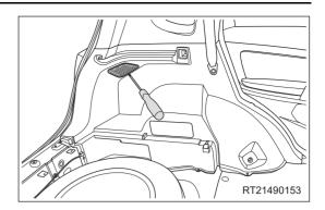
g. Remove 5 fixing screws (arrow) from the C-pillar lower protector assembly.
