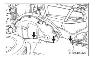
e. Remove the clips (arrow) on the rear part of fuel filler cap cable and remove the fuel filler cap cable.
