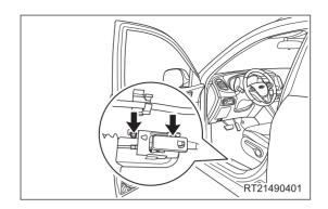
b. Remove the fuel filler cap cable from the fuel tank opening bracket assembly in the direction of arrow as shown in the illustration.
