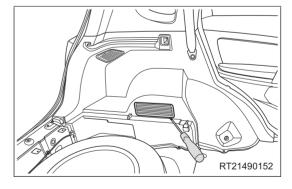
f. Using a screwdriver wrapped with protective tape, pry off the rear combination light service cover and remove the rear combination light service cover.
