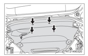
b. Take out the roof assembly from the back door.
