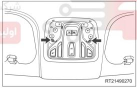
c. Remove the front dome light assembly.
