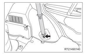
b. Remove the warning triangle box (for right side) in the direction of arrow as shown in the illustration.
