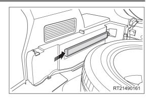
c. Using a screwdriver wrapped with protective tape, pry off the back door light cover (for right side).
