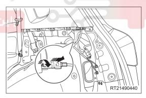
d. Remove the clips (arrow) on the side of fuel filler cap cable.
