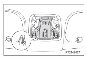
d. Disconnect the interior front dome light connector (arrow), and remove the interior front dome light assembly.
