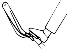
2. With the engine stopped, step on the brake pedal several times.
