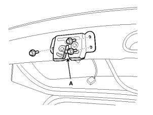
3. Disconnect the tail gate latch connector (A).
