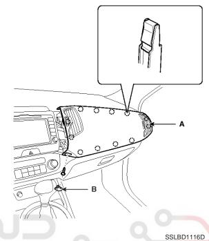
6. After loosening the mounting screws, then remove the center facia panel (A).
