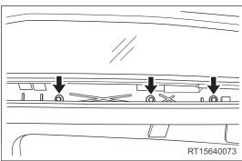
c. Remove the sliding roof rear glass.
