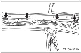
f. Remove 4 fixing bolts (arrow) between right side of sliding roof fixing bracket and roof.
