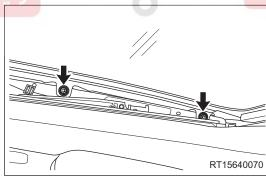
c. Remove the sliding roof front glass.
