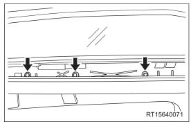
b. Remove 3 fixing bolts (arrow) from right side of sliding roof rear glass.
