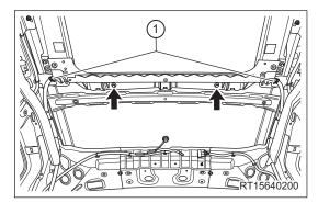
e. Remove 4 fixing bolts (arrow) between left side of sliding roof fixing bracket and roof.
