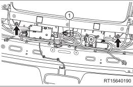
d. Loosen the sliding roof glass rear drain hose fixing clamps (1) and the 2 fixing bolts (arrow) between rear end of sliding roof fixing bracket and roof.
