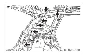
b. Detach lower part of sliding roof rear drain hose from fixing sponge (arrow).
