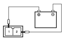
**CONDENSER FAN RELAY (Type A)** Check for continuity between the terminals.
