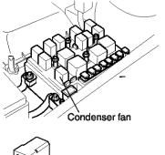
1. There should be continuity between the No.87 and No.30 terminals when power and ground are
