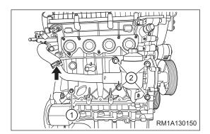
f. Remove water pump and cooling pipe assembly I from oil filter module.
