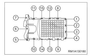
c. Pry oil pan at specific prying locations on oil pan with oil pan remover and scraper to remove it.
