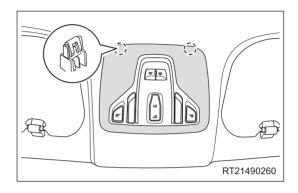
b. Remove 2 fixing screws (arrow) from roof switch set. (Tightening torque: 1.5 ± 0.5 N⋅m)
