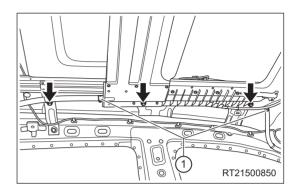
Remove 3 fixing bolts (arrow) on the right side of the sliding roof bracket, loosen the 2 clamps (1) and disconnect the right side drain hose.
