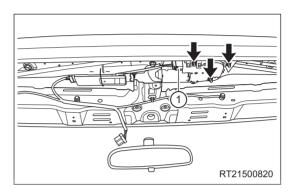
b. Remove the roof motor.
